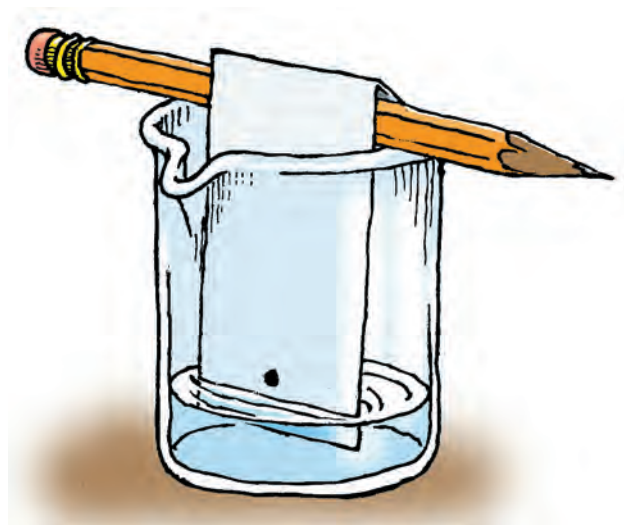
Figure 17.2 Use a pencil to hang the paper in the beaker containing the water. Make sure the ink spot is above the surface of the water.
