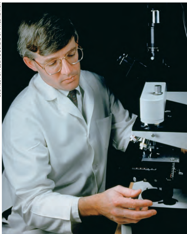
An FBI special agent uses a comparison microscope to compare fibers from a crime scene with those from the carpet in a suspect's car (above right).
