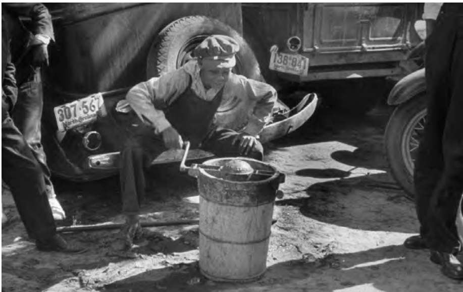
This ice cream machine required the use of ice and salt to lower the temperature of the ice cream mixture to the point where it would freeze.
