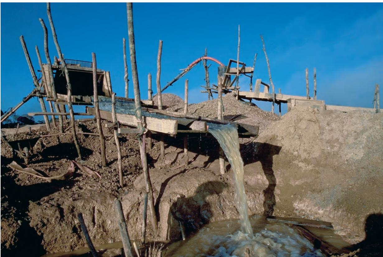
*This sluice is being used by prospectors in Amazonia to separate gold from water and mud.*
