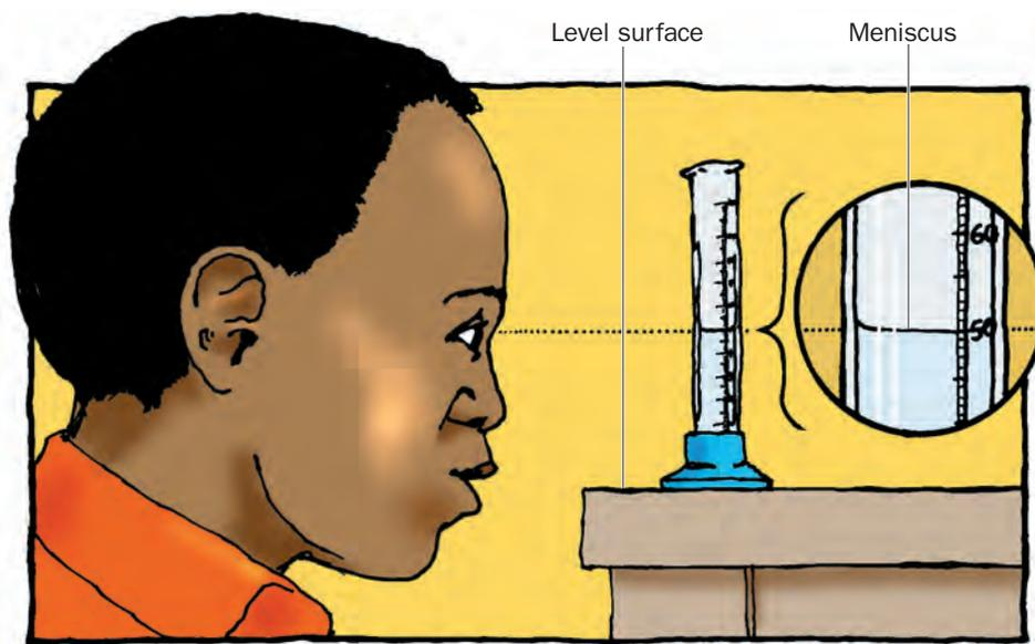
**Figure 2.2** Make sure the graduated cylinder is on a level surface. When you take a reading, make sure your eye is level with the bottom of the meniscus. The “meniscus” is the curved upper surface of the water in the cylinder.
