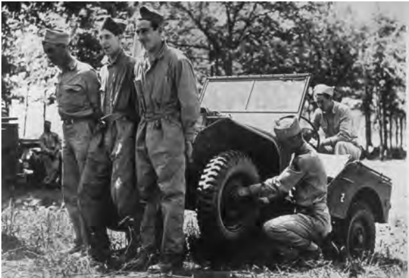
When the Japanese army took over the rubber plantations in the Far East, rubber was in short supply. The tires on this army truck were made from a new plastic, sometimes called synthetic rubber.
