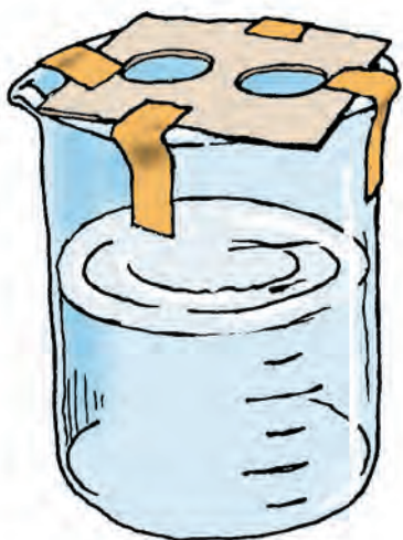
Figure 22.2 Use tape to affix the index card to the top of the beaker.
