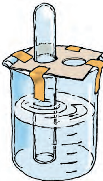
Figure 22.3 Place an empty test tube through the index card, with the open end of the test tube resting on the bottom of the beaker.
