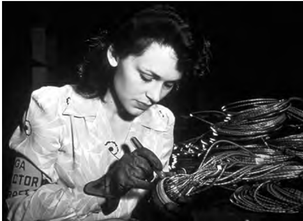
Polyvinyl chloride (PVC) was used to insulate electrical wires inside aircraft.
