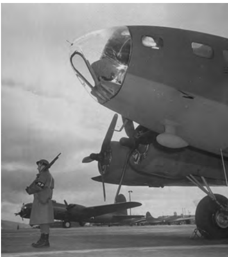
Polyacrylics (for example, Plexiglass™) were transparent and light and didn't shatter like glass—ideal properties when it came to aircraft manufacture.
