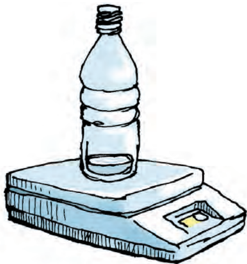
Figure 25.2 After the reaction has stopped, measure the mass of the bottle, its cap, and its contents, keeping the cap tightly sealed.
