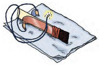
Figure 2.6 Lay the zinc-copper assembly on a paper towel.
