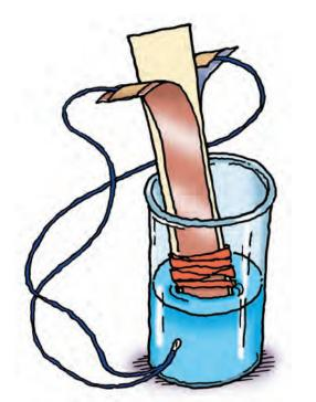
**Figure 2.5** *Place the zinc–copper assembly in the copper sulfate solution.*
