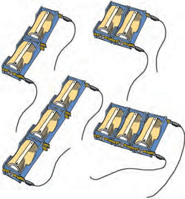
Figure 7.2 Some possible ways to connect the batteries
