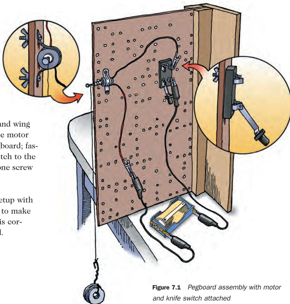
**Figure 7.1** Pegboard assembly with motor and knife switch attached
