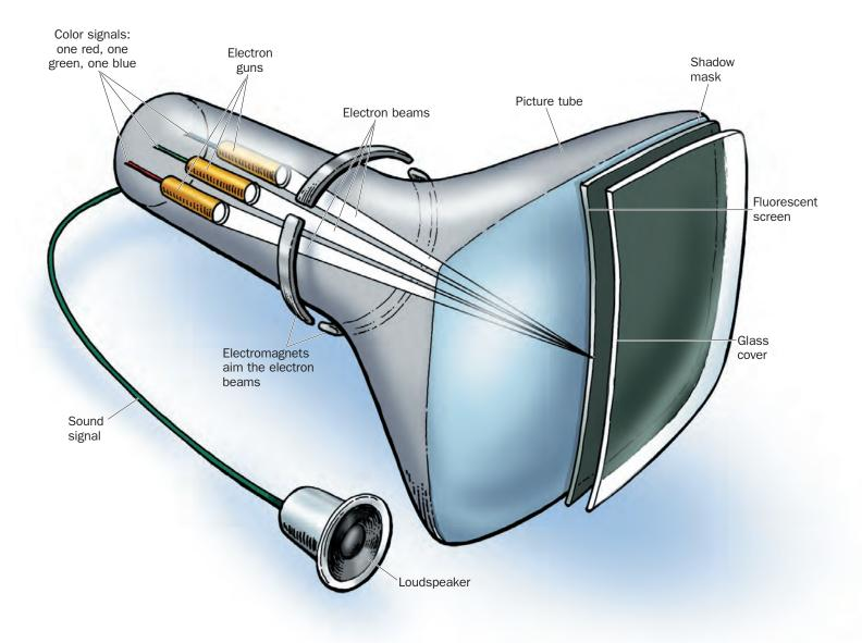
Inside a TV set, there are three electron guns, one for each color. These guns fire beams of electrons that make the red, green, or blue pixels glow to form a picture of many colors by using additive color mixing. The guns scan alternate lines of pixels that make up each picture. Each picture is therefore scanned onto the screen twice—60 scans or 30 complete pictures each second.
