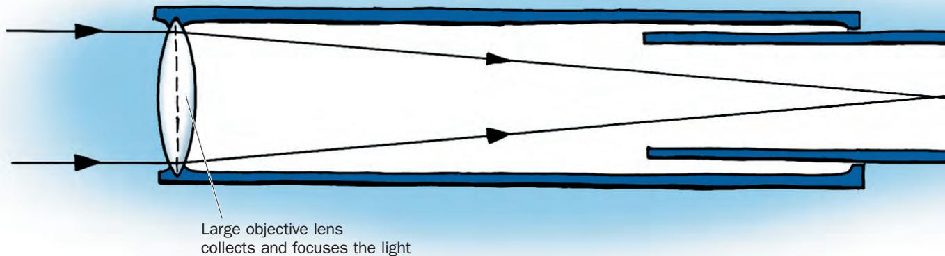
*The components of a simple refracting telescope. This type of telescope is often referred to as a Keplerian telescope because it was used by the famous astronomer Johannes Kepler (1571–1630). Is the image produced by this telescope upright or inverted?*
